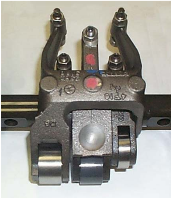
DDC Series 60 Rocker Arm Assembly with Ceradyne's Ceralloy® 147-31N Silicon Nitride Cam Roller
