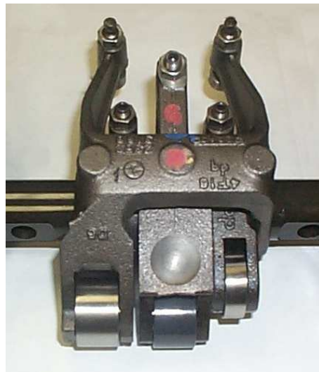
DDC Series 60 Rocker Arm Assembly with Ceradyne's Cerallloy® 147-31N Silicon Nitride Cam Roller
