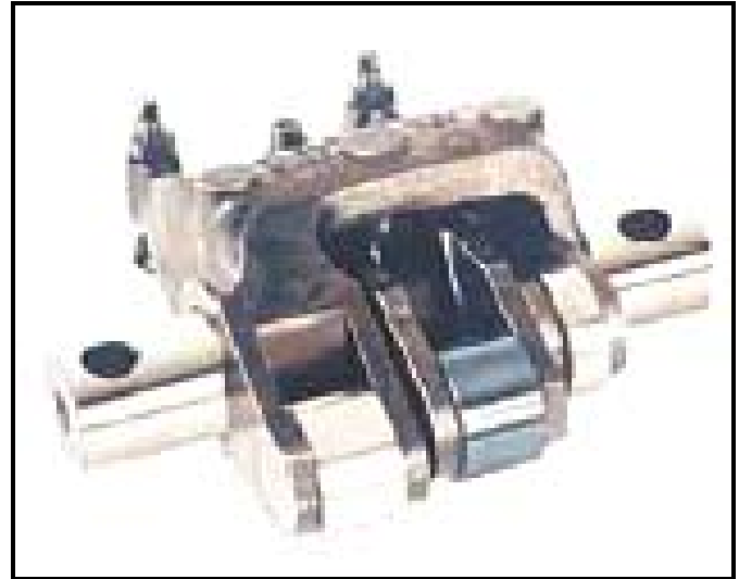
Figure 2. DDC Series 60 rocker arm assembly with a Si 3 N 4 cam roller follower (dark gray) in the fuel injector position, allowing fuel injection pressures of over 210 MPa (30 ksi) 10 .
